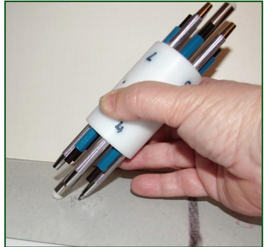
If crushing of the hardest lead should occur, the film is extremely hard, and is beyond the measuring range of the device. If scratching or marring of the film occurs, proceed with the next softer lead grade and repeat the testing procedure until a test lead is found that crushes and does not mar the film. Confirm the result with duplicate observations of the last (crushing) lead, and the next hardest (marring) lead.
