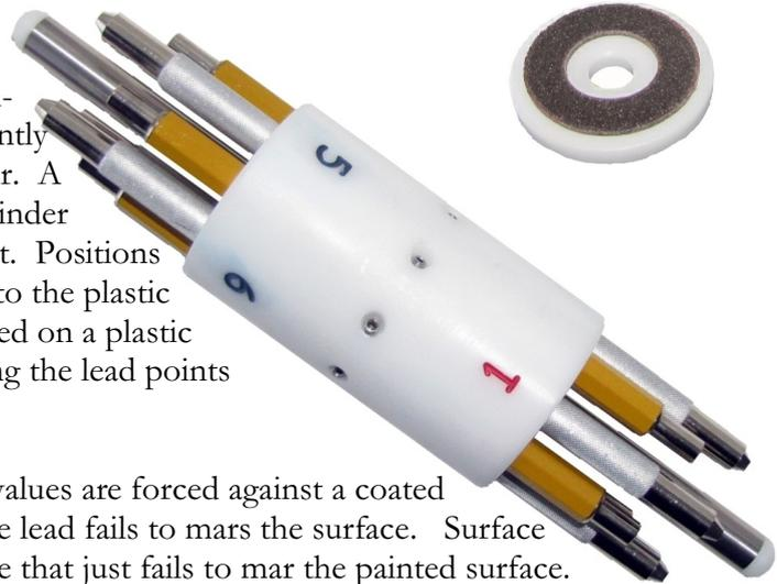
In a test, pencil leads of decreasing hardness values are forced against a coated surface in a precisely defined manner until one lead fails to mar the surface. Surface hardness is defined by the hardest pencil grade that just fails to mar the painted surface.
