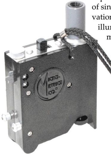
A precision tool for inspection and thickness measurement (ASTM D4138) of single or multiple coats on any substrate, and for microscopic observation and measurement of substrate and film and film defects. Uses an illuminated 50-power microscope with a "universal" measuring reticle that measures in mils, microns, and millimeters; and mounts three tungsten-carbide cutting tips for precise incision of the surface.
