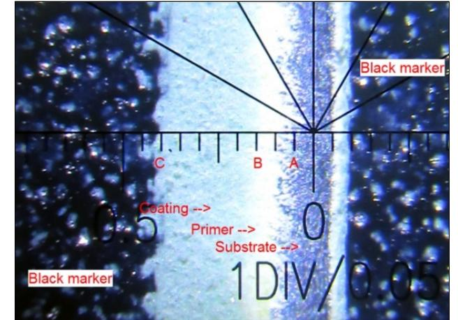
(Measuring: Line "A" marks the edge between substrate and primer. Line "B" is the line between primer and top-coat. Line "C" is the top of the coating, made easier to see by using the black marker. View through the universal scope.)
