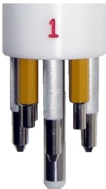
The Micro-Metrics H-501 Pencil Hardness Gauge is unique in that it provides a compact single unit for performing the testing, rather than a set of easily lost individual lead holders. The importance of this difference should not be discounted, especially when several individuals may be working with a single instrument, or when the testing must be done in awkward or difficult situations, where swapping out single lead holders may result in dropping one.
