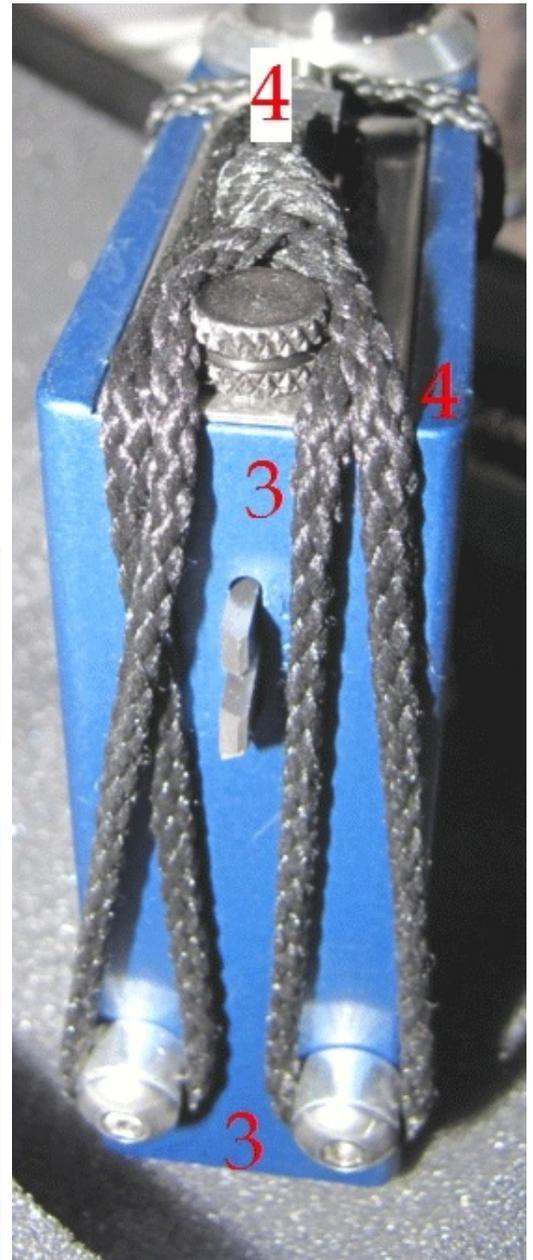
These steps make it easier to fit the Tooke Gage into the foam insert in the carry case, and prevents the switch from accidentally turning on while the case is closed.
