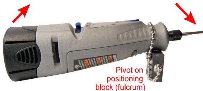
Figure 2. Positioning block shown for the 1x cutting angle.
