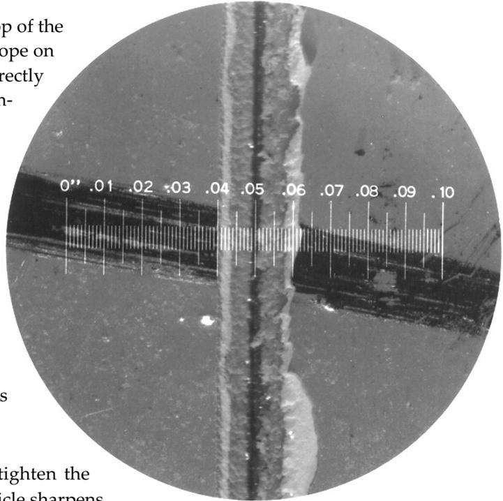
**Note:** If the reticle seems out of focus, unscrew or tighten the chrome eyepiece of the microscope slightly, until the reticle sharpens.
